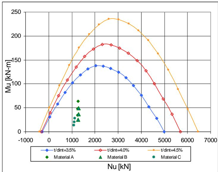
Figure 7. Interaction diagrams for lining with internal diameter of 6.0m.
