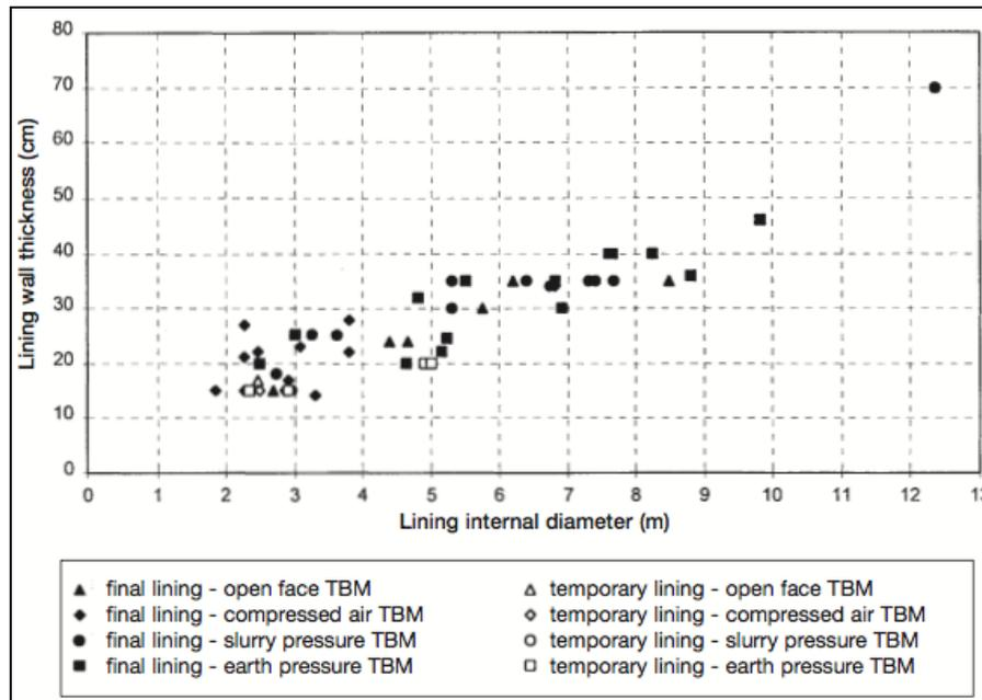
Figure 2. AFTES worldwide data compilation of the ratio between lining wall thickness and tunnel internal diameter. Reproduced from [2].
