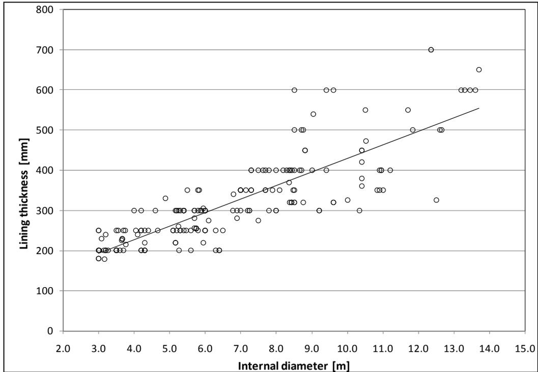
Figure 3. Compilation of lining thickness and internal diameter of tunnel projects around the world.
