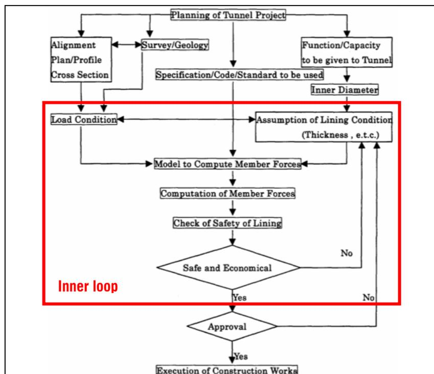
Figure 1. ITA flow chart for segmental lining design. Reproduced from [3].
