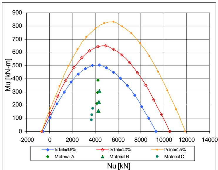
Figure 9. Interaction diagrams for lining with internal diameter of 11.0m.
