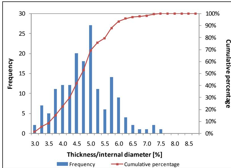
Figure 5. Histogram and cumulative percentage curve of thickness/internal diameter data for tunnels with internal diameters larger than 4.5m.
