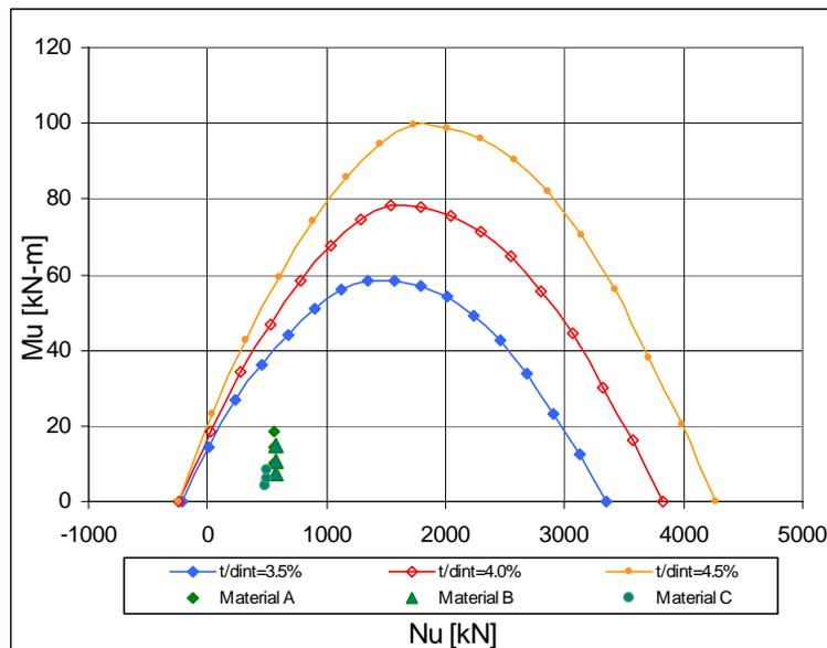
Figure 6. Interaction diagrams for lining with internal diameter of 4.0m.
