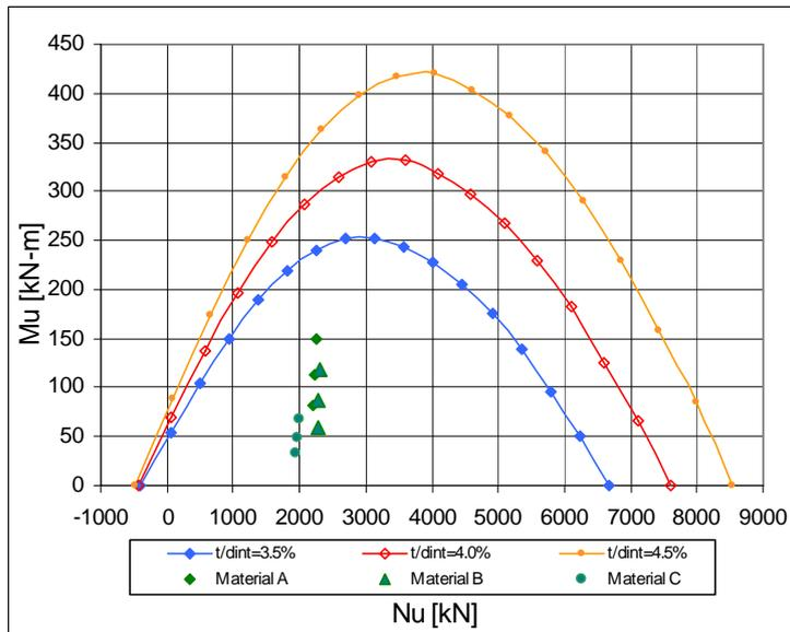
Figure 8. Interaction diagrams for lining with internal diameter of 8.0m.
