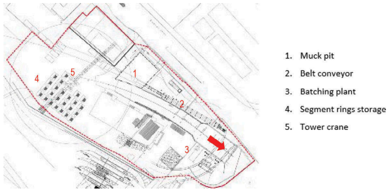
Figure 5. TBM launching site layout.
